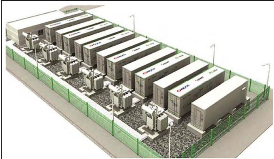
Figure 7-2: Typical illustration of a Battery Energy Storage System Technology
