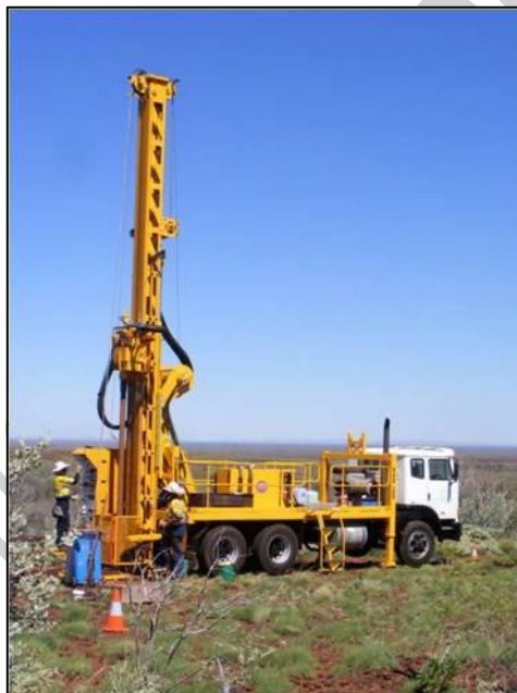
Figure 4: Example of a Typical Drill Rig
