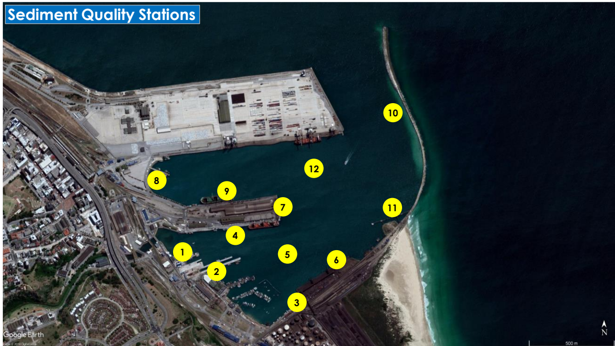
Figure 32: Aerial view of the Port of Port Elizabeth showing the positions where sediment was sampled in surveys between 2015-2019 for the Long-Term Ecological Monitoring Programme.
