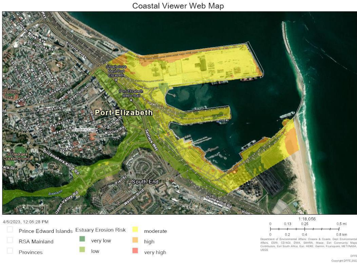
Figure 54: Estuarine erosion risk profile of Old Tug Jetty (DFFE O&C. 2023)
