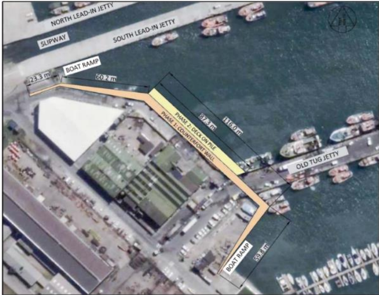
Figure 4: Phase construction of preferred solution
