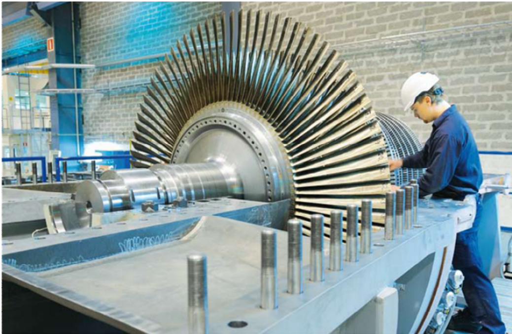
Figure 2.3: The steam turbine rotor, primary component of a steam turbine (Source: Siemens AG).
