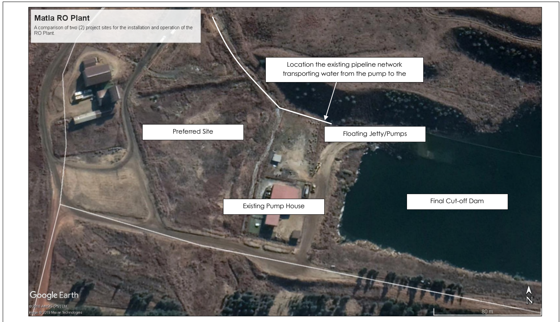
Figure 2.5: A satellite image illustrating the proximity of the preferred project site to the existing pump station, the Final Cut-off Dam where the required water will be sourced from and the existing pipeline network required for the transport of the permeate flow back to the station.
