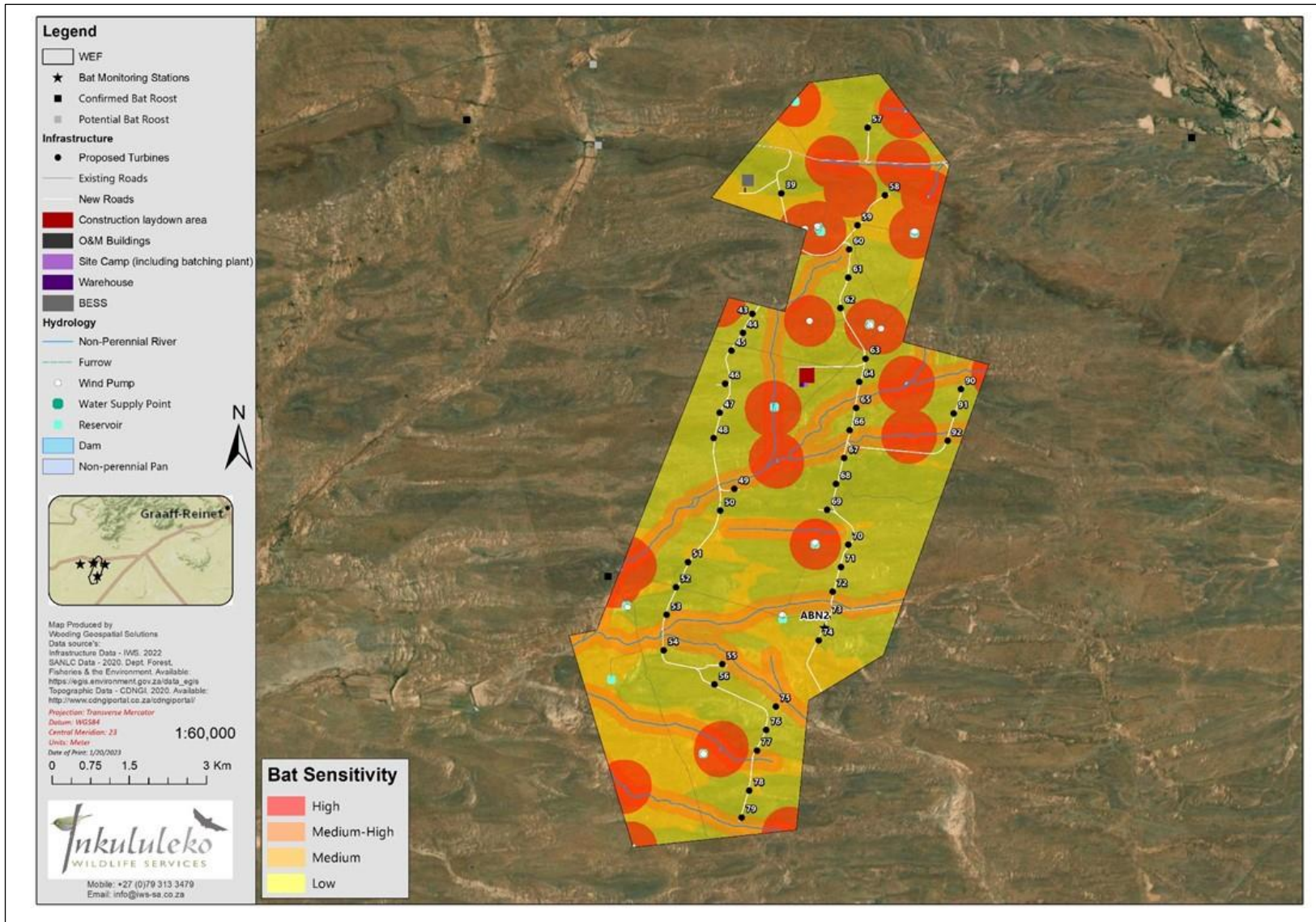
Figure 9.6: Bat sensitivity map showing all no-go area buffers which needs to be considered for the placement of wind turbines
