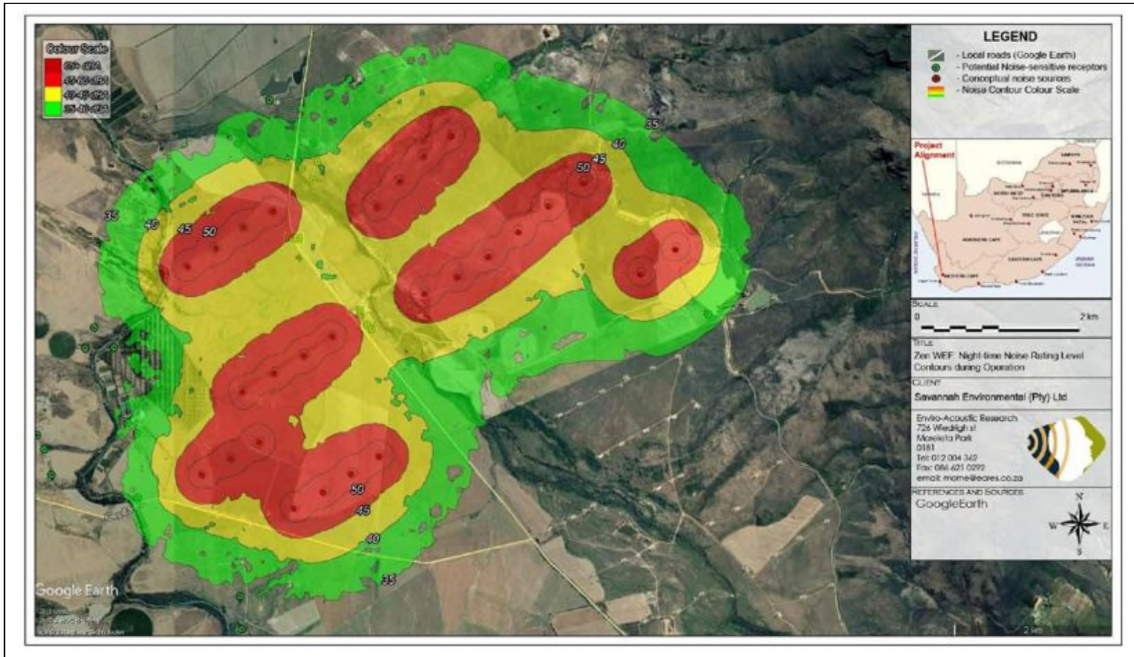
Figure 5.4: Noise rating level contours as modelled for the Zen Wind Energy Facility.
