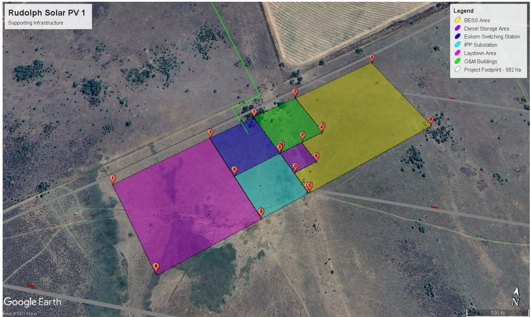
Figure 1.2: Co-ordinate points of supporting infrastructure
