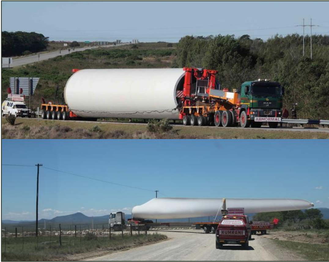
Figure 5.9: Tower section in low load configuration shown in top photo; and blade shown in bottom photo
