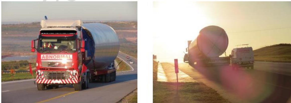
Figure 8: Example - transport of tower sections (JG Afrika, April 2022)
