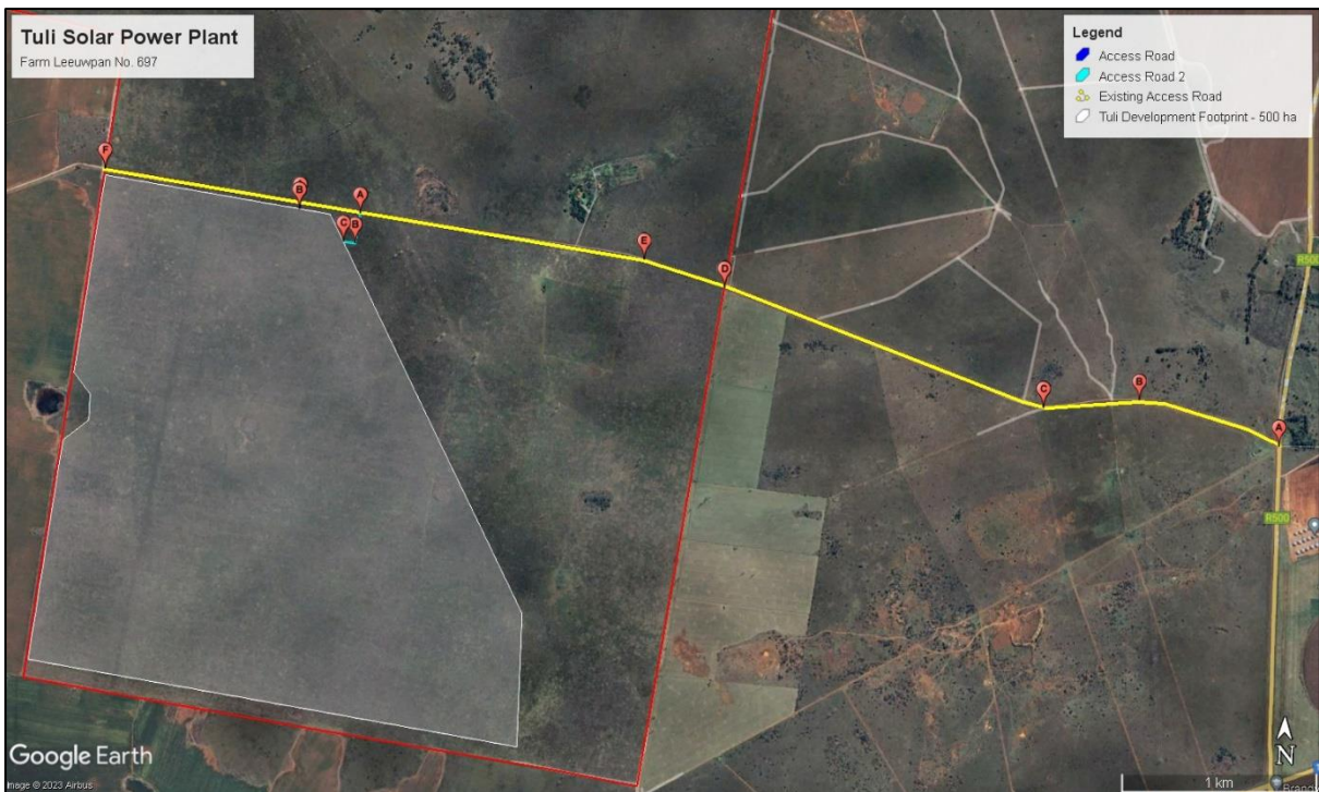
Figure 2.3: Map illustrating coordinate points of the proposed access road 1, access road 2 and the existing access road from the R500 for the Tuli Solar Power Plant.
