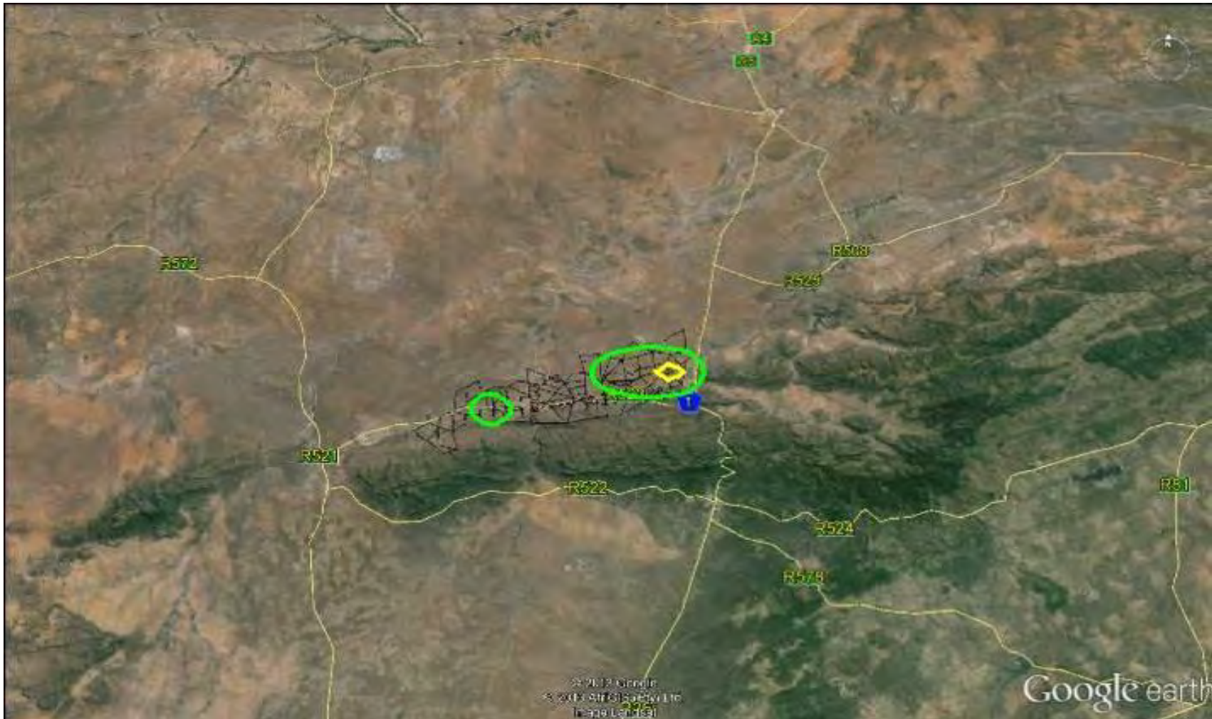
Figure 94: Dust fallout impacts recorded during the operational phases of the Chapudi Project (Yellow: 300 mg/m 2 /day, Green: 600 mg/m 2 /day)
