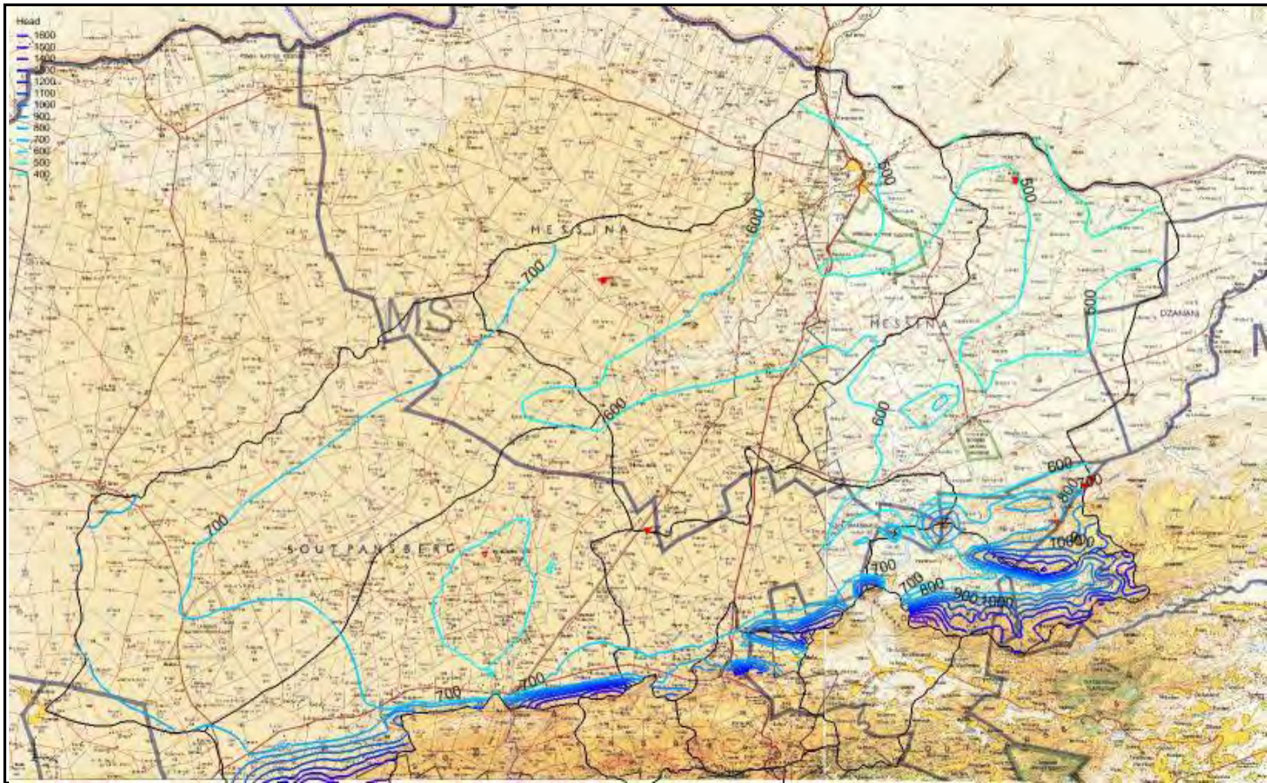
Figure 40: Steady state water levels under current conditions (metres above mean sea level)
