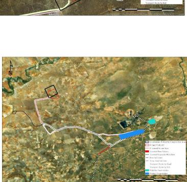
Product will be transported from Monday through to Sunday during daylight hours. The mine will require thirty-six (36) 50-tonne side tipping trucks to transport 10,000 tonnes per day calculated at 5.5 x truck loads per vehicle per day. Alternatively, the product can be transported to the Temo Railloop Rapid Load-Out Facility planned approximately 400m south of the CHPP on farm Duikerpan 249 LQ (still
