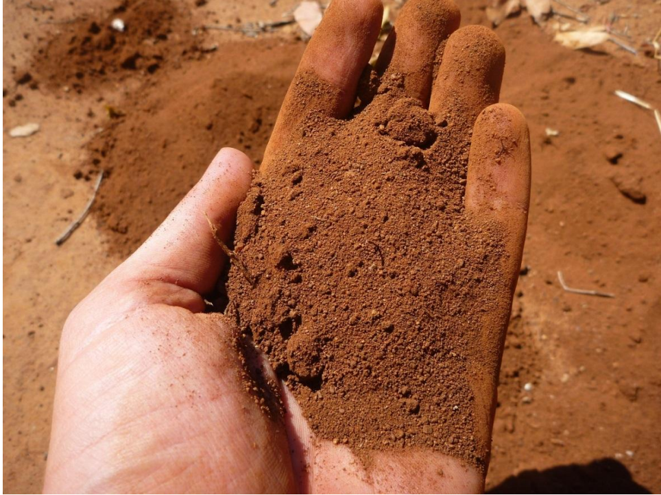
Figure 17 The red colouration of the red apedal B-horizon of the soils of the Hutton soil form is ascribed to hematite dominating the Fe oxide mineral phases
