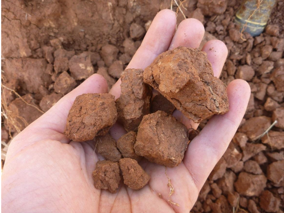
Figure 20 The blocky structure of the vertic A-horizon exhibiting pressure faces and slickensides
