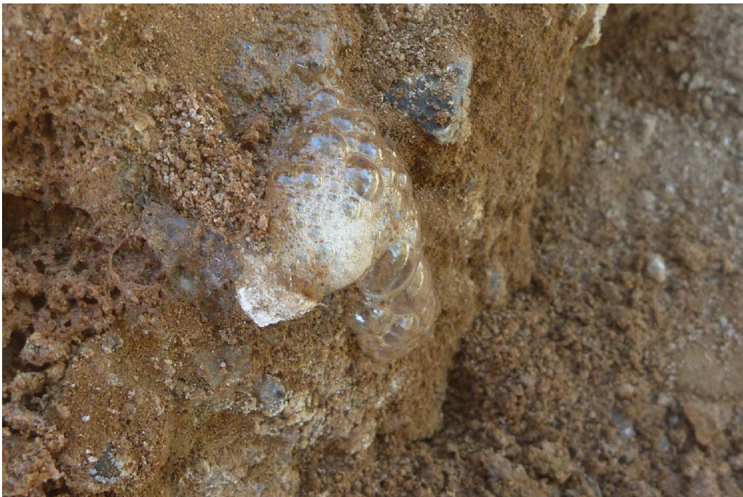
Figure 13 Fizzing of calcium and/or potassium–magnesium carbonates when reacted with a 10 % HCl solution
