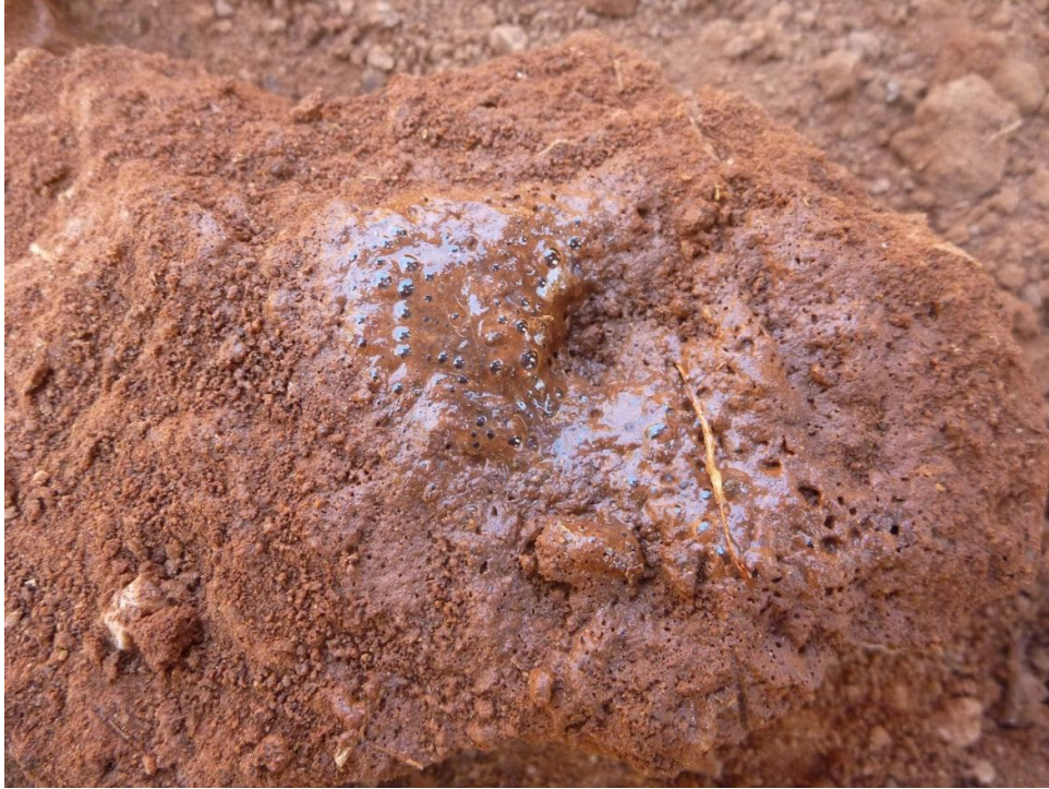
Figure 15 The neocutanic carbonate B-horizon, although not morphologically dominated by carbonates, fizzes when reacted with a 10 % HCl solution
