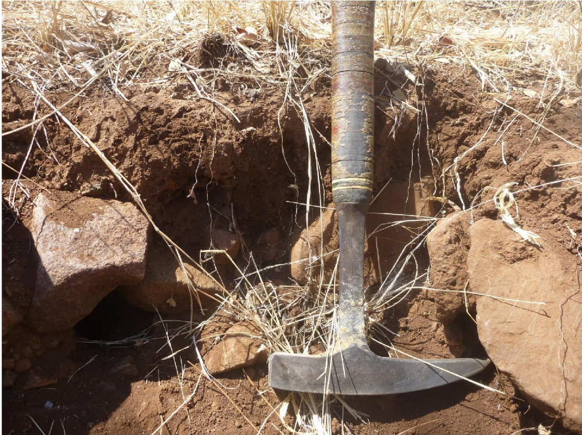
Figure 10 Soil of the Mispah soil form which occur in the higher lying areas of the site (polygon 13)
