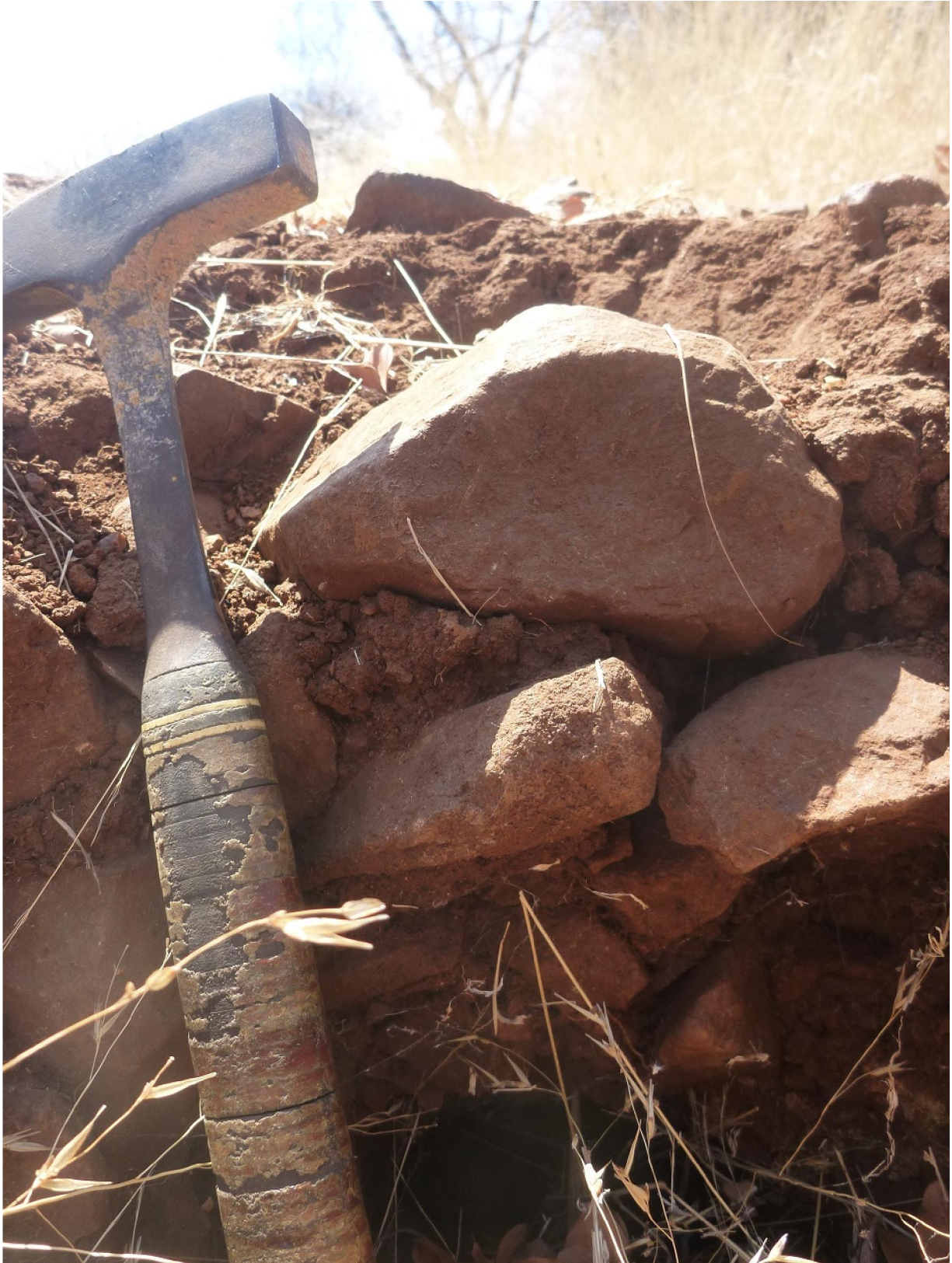
Figure 8 Augering depth is shallow in the area described as soil-rock complexes (polygon 13) for the study area owing to the rockiness of the soils
