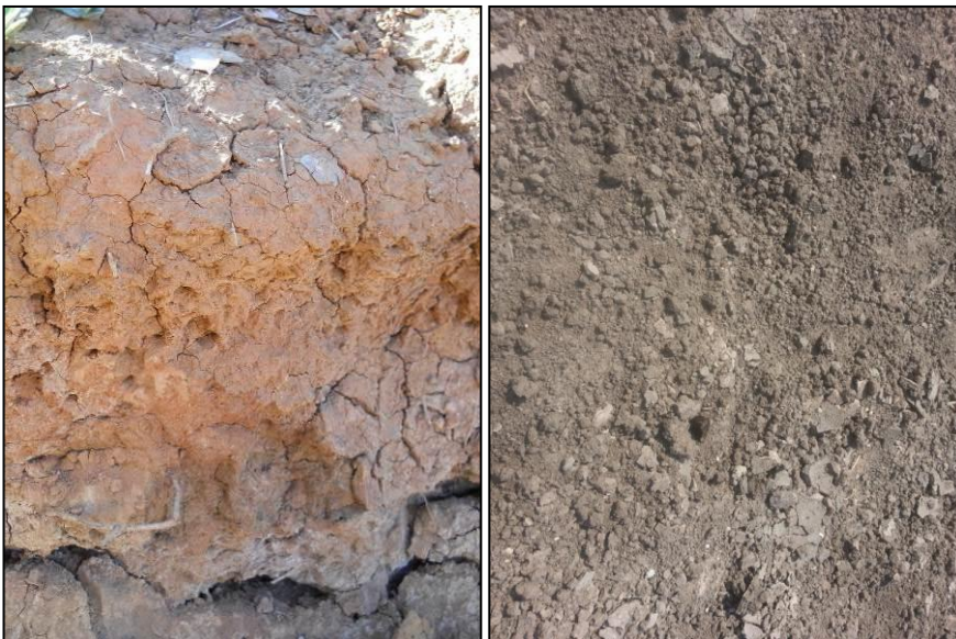
Figure 47: Gleying evident within the soil profile of the smaller drainage lines with riparian zones (left); gleyed soils within the permanent zone of pans (right).
