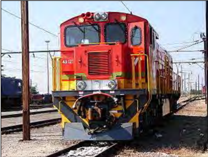
Figure 4-2: Class 43 diesel locomotives
