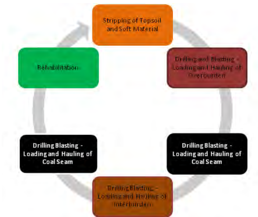
Figure 1.3: Schematic presentation of the mining process
