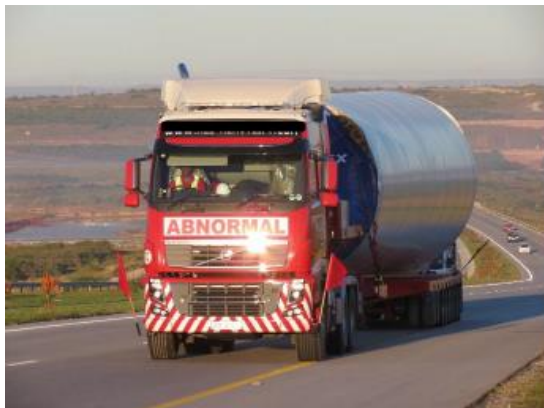
Figure 8: Example - transport of tower sections (JG Afrika, April 2022)
