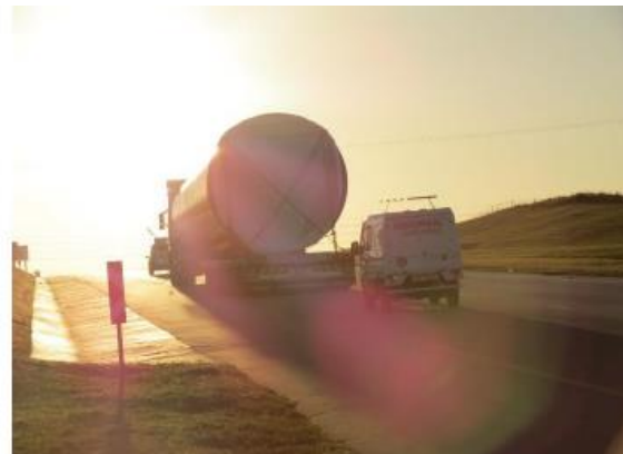
Figure 8: Example - transport of tower sections (JG Afrika, April 2022)
