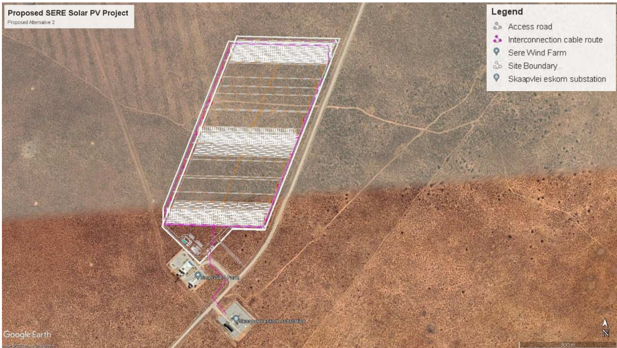
Figure 12: Map of Alternative 2 showing both the fixed and tracking layout options (Google Earth image)
