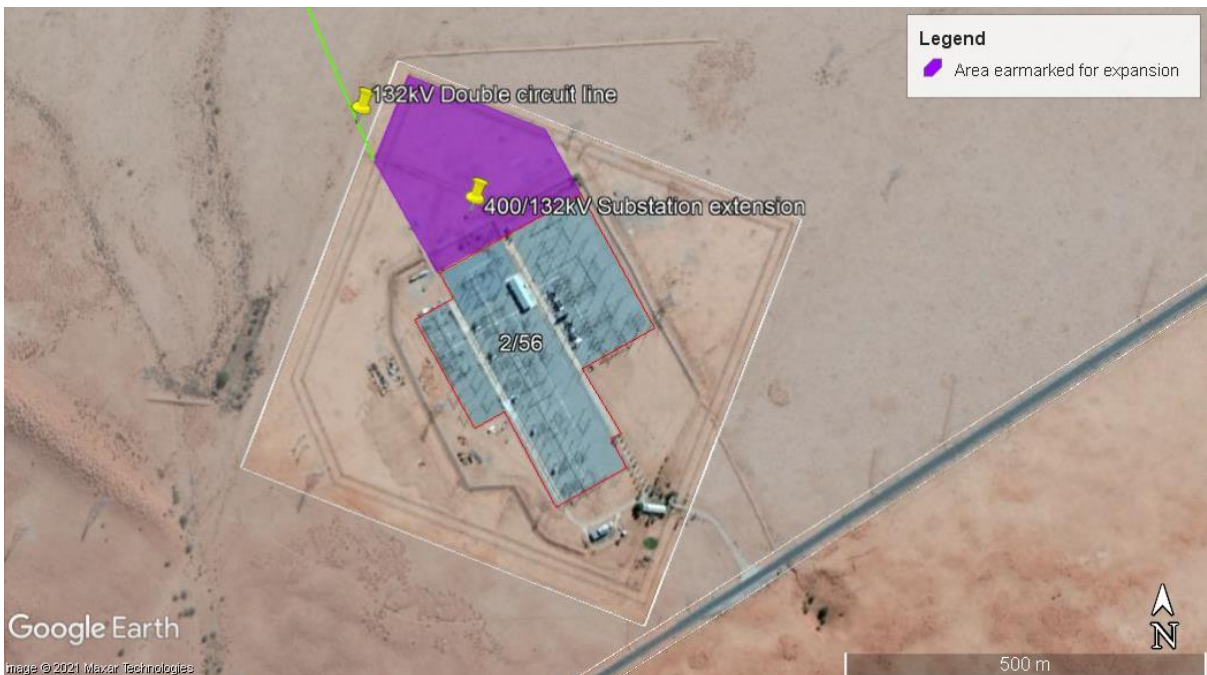
Figure 2: Area earmarked for the expansion of the Aggeneys substation
