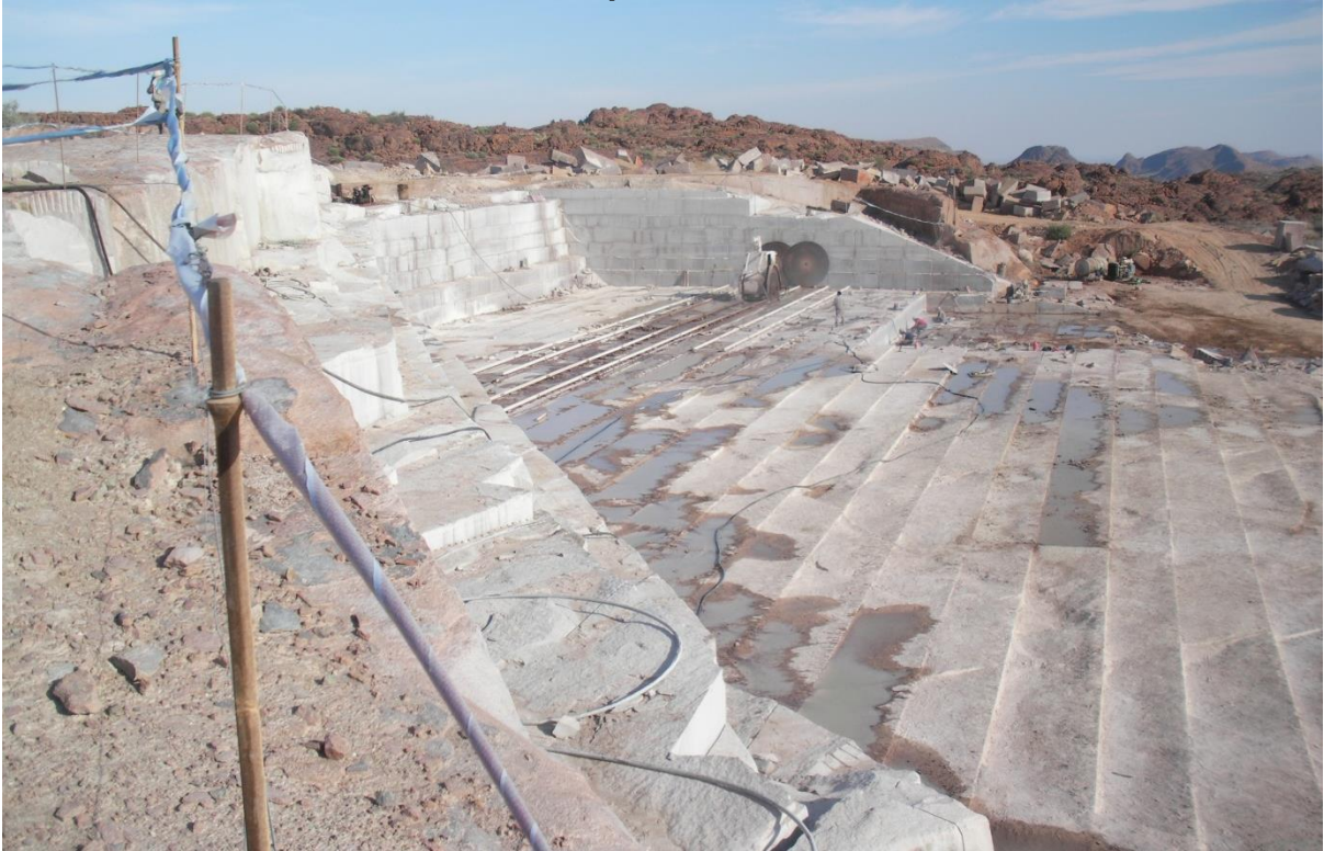
Photo 2 Circular saw with tracks being laid
