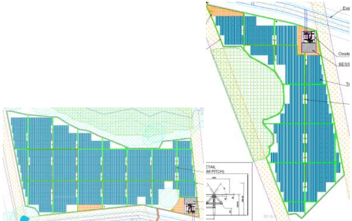
Figure 18: Perimeter and internal roads (green) for Roan 1 PV North (left) and Roan 1 PV East (Right)
