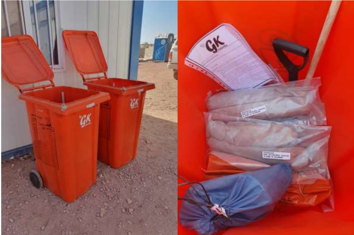
Figure 23: Hydrocarbon Spill Kits must be in place within the site camp and in the field within 500 m of any drilling or ramming activity.
