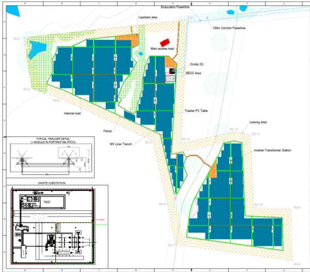
Figure 2: Proposed layout of Roan 2 PV, showing key project components (Please also refer to the full-scale plans attached in Appendix D).
