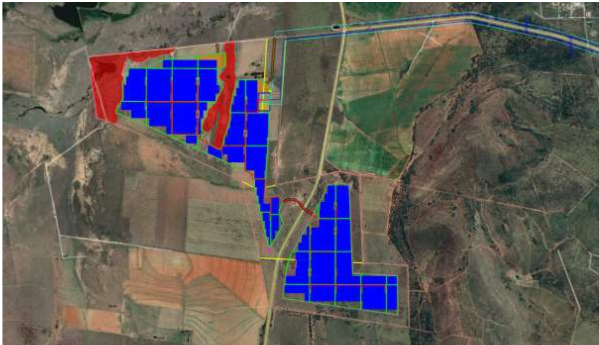
Figure 62: Roan 2 PV Showing the exclusion of the identified ecologically sensitive areas and associated buffers.
