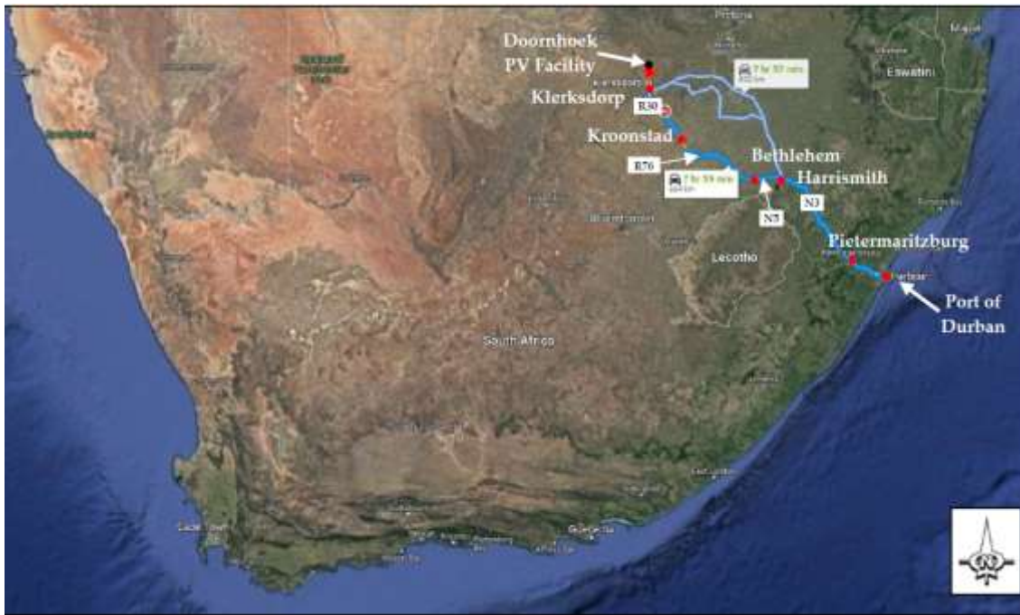
Figure 12: Preferred Transport Route from Durban Harbour to Doornhoek 1 PV facility (BVi Consulting Engineers, 2022).
