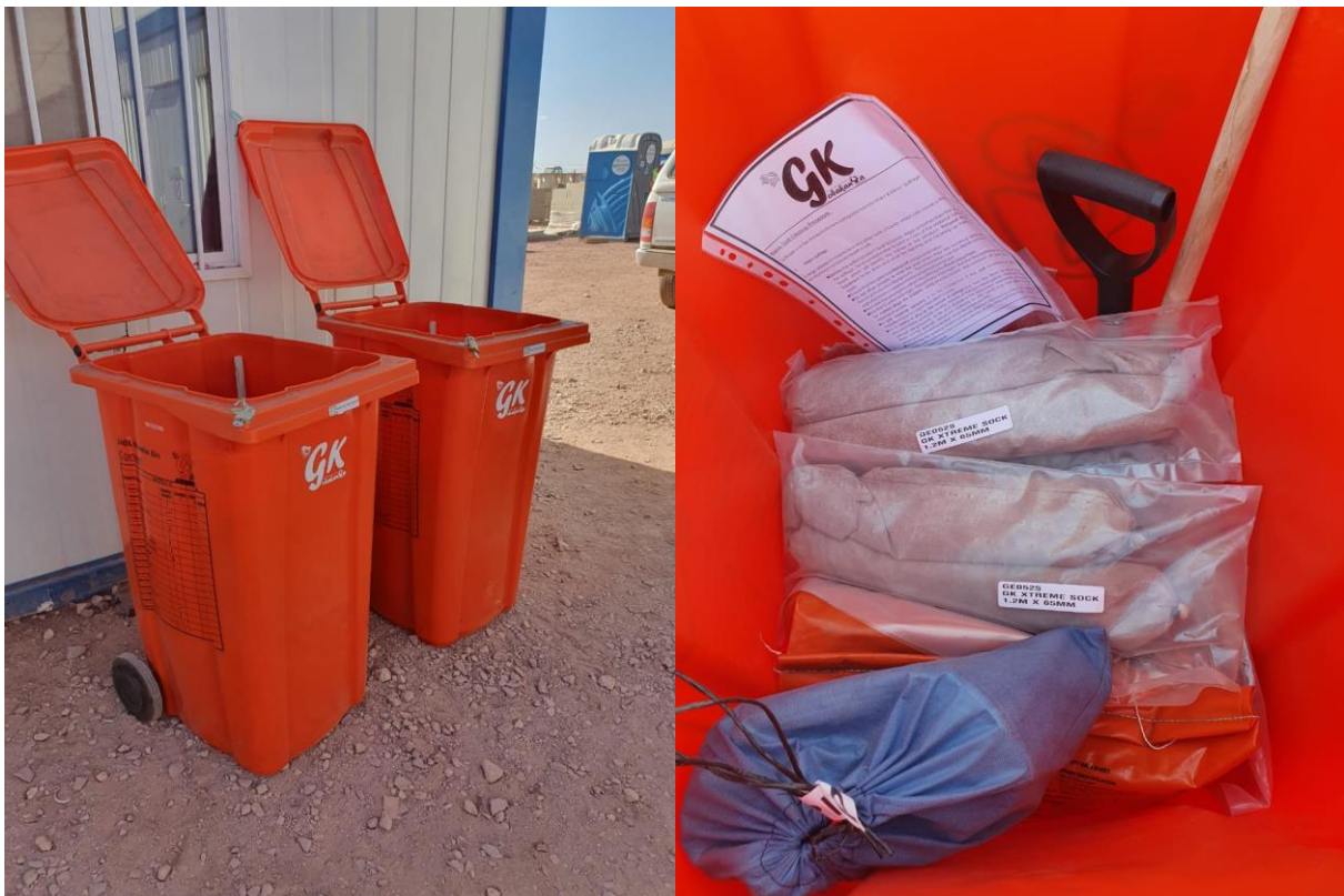
Figure 13: Hydrocarbon Spill Kits must be in place within the site camp and in the field within 500 m of any drilling or ramming activity.
