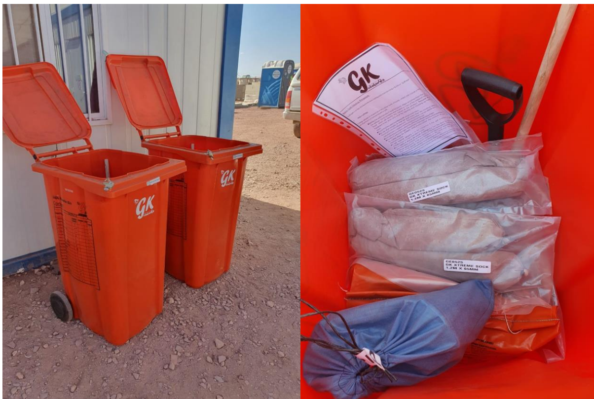
Figure 15: In compliance with the EMPR (Appendix H) Hydrocarbon Spill Kits must be in place within the site camp and in the field within 500 m of any drilling or ramming activity.
