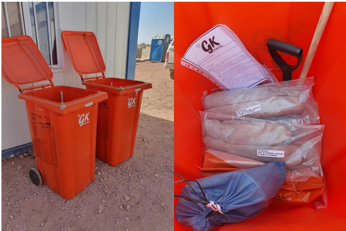
Figure 15: In compliance with the EMP (Appendix H) Hydrocarbon Spill Kits must be in place within the site camp and in the field within 500 m of any drilling or ramming activity.
