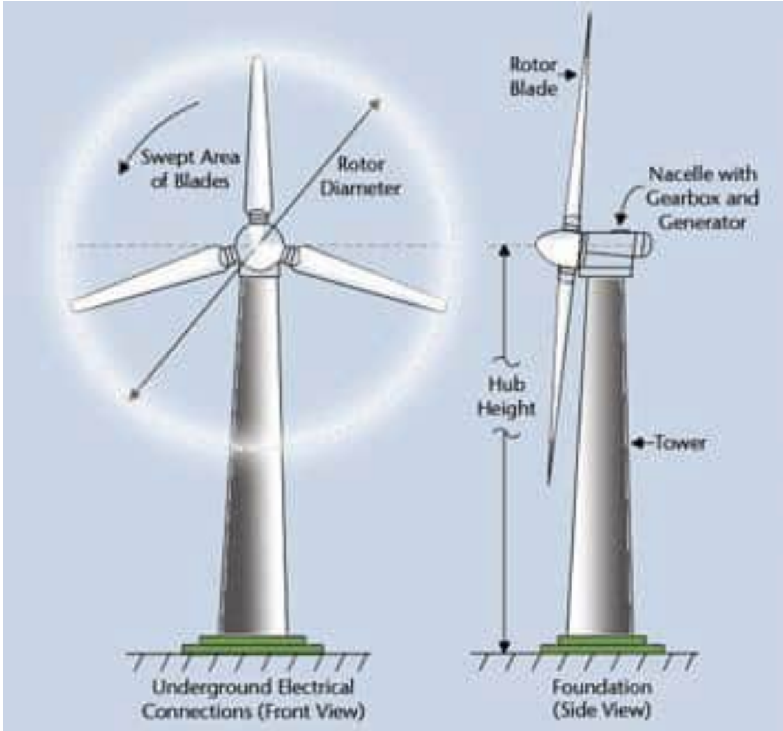
Figure 6-5 - Illustration of the main components of a wind turbine
