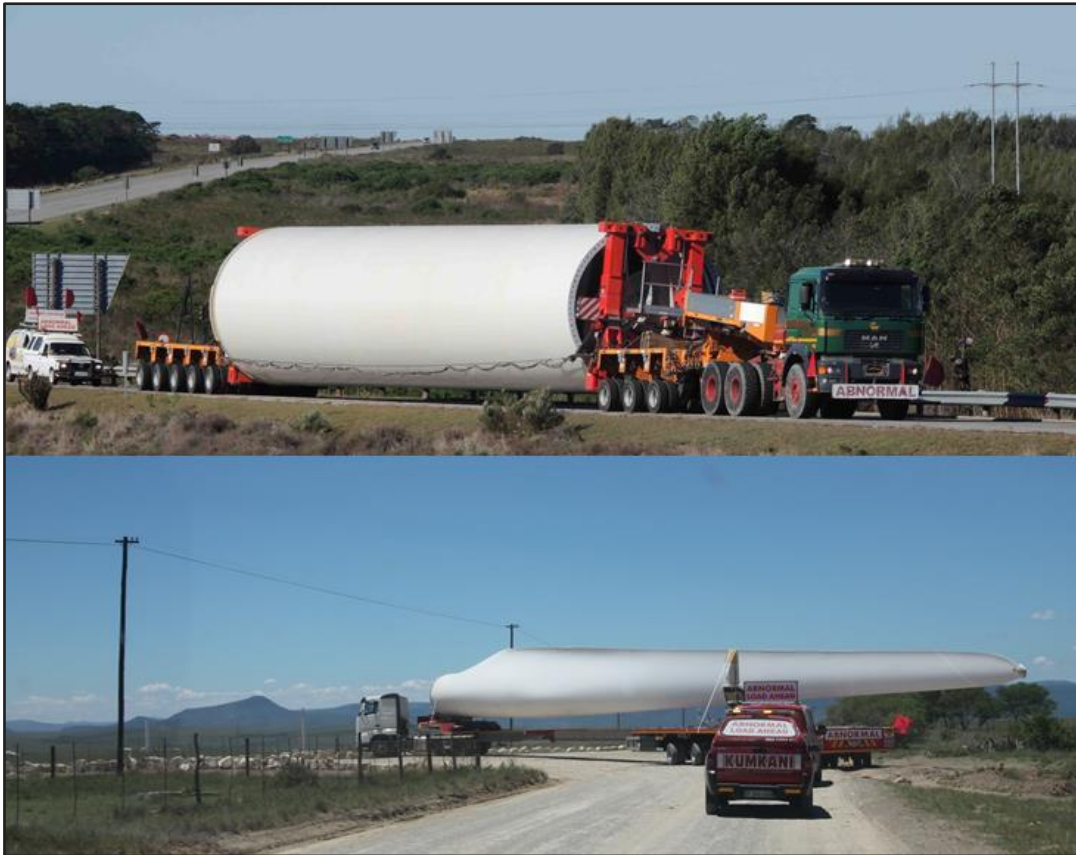
Figure 5-5 | Abnormal freight (tower section in low load configuration (top) and blade (bottom))
