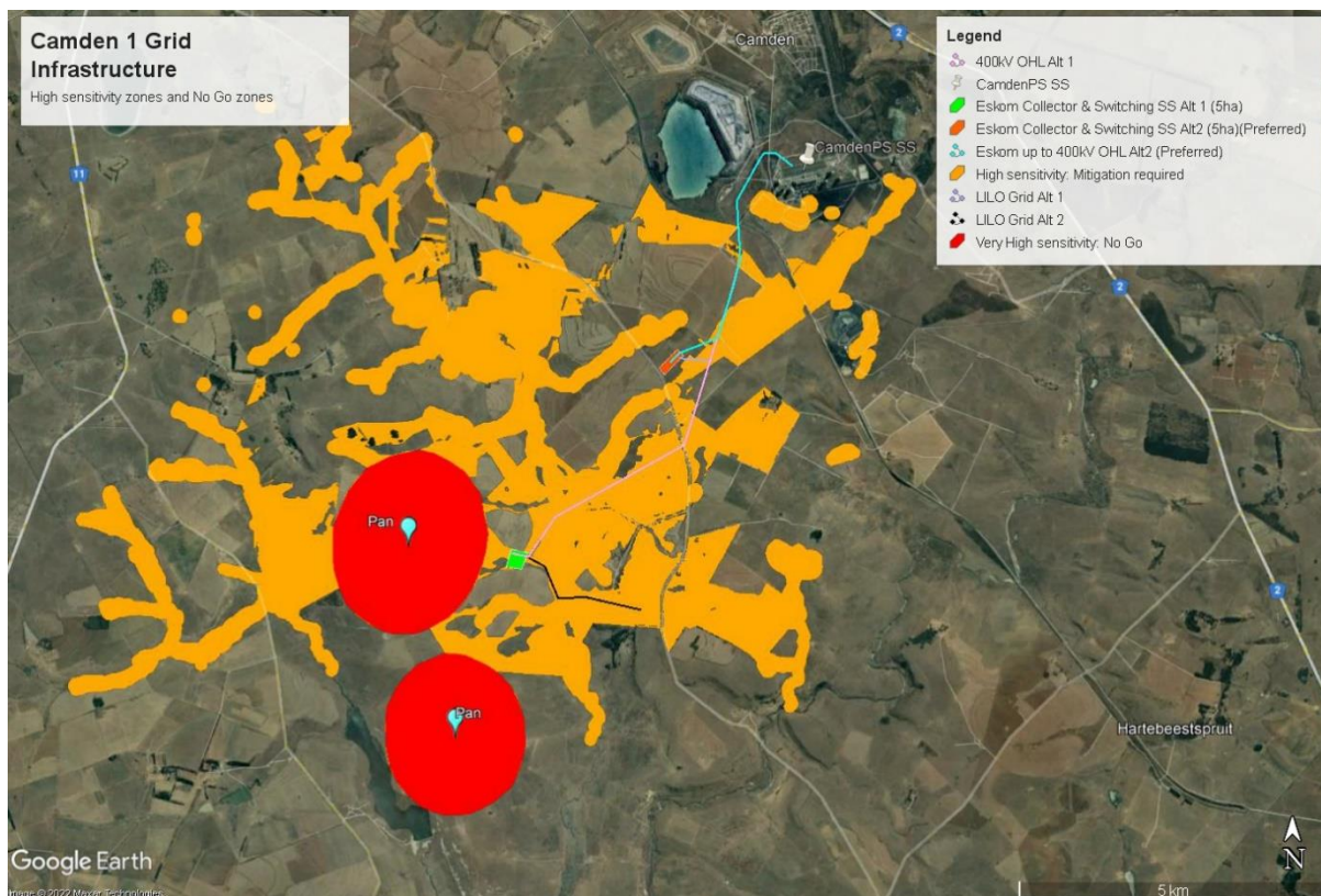
Figure 5-20: Proposed avifaunal sensitivities for the 400kV Grid Infrastructure (red zones around the pans) (Chris van Rooyen Consulting, 2021).
