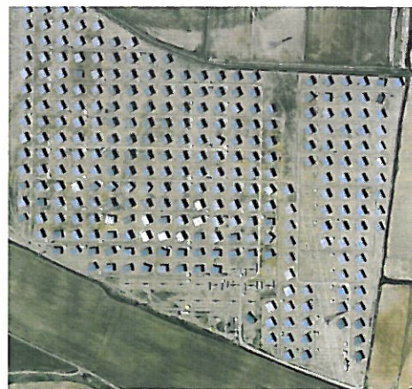
Figure 4 –Typical CPV Facility Layout
