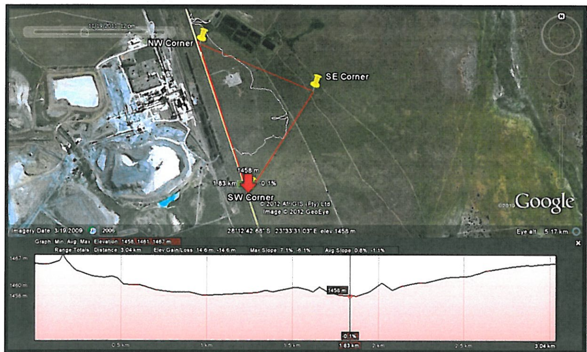
Figure 7 – Google image indicating the slope following the boundary of the site (direction NW -SE-SW).From Fig 5 of Biodiversity Assessment; Appendix D2.
