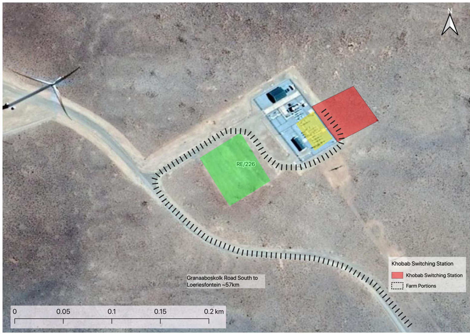
Figure 5-1: Proposed Khobab switching station in red (eastern side of the existing Khobab Substation), yellow square indicates area where switching station will connect to substation, green square indicates potential laydown area (previously cleared), existing access route indicated by hashed line.
