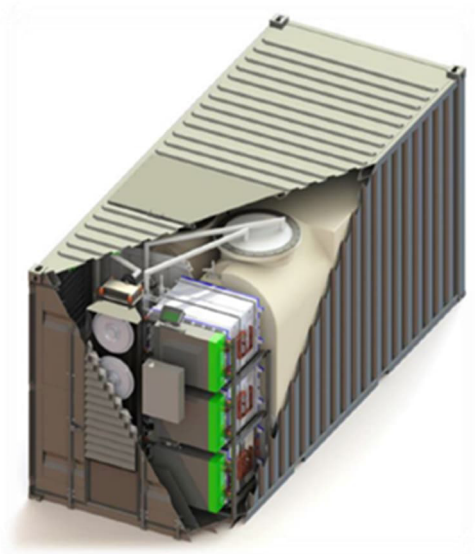
Figure 3-6 Typical Storage of Flow Batteries
