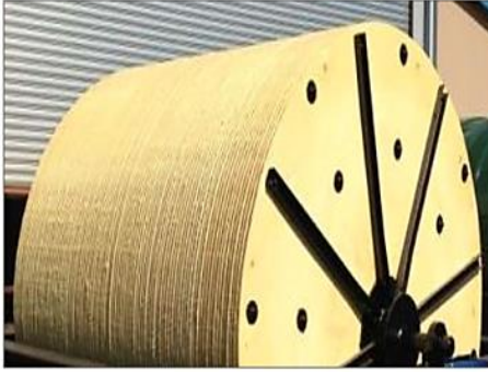
Figure 4-7: Illustrative representation of Rotating Biological Contactors
