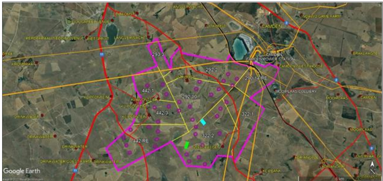
Figure 6-44: Camden I WEF site (pink) and substation/BESS Alt 1 (green fill) and Alt 2 (blue) in relation to site properties (yellow). Pink circles indicate proposed turbine locations. Also indicated are existing power lines (orange), the railway line (black) and local road network (red)
