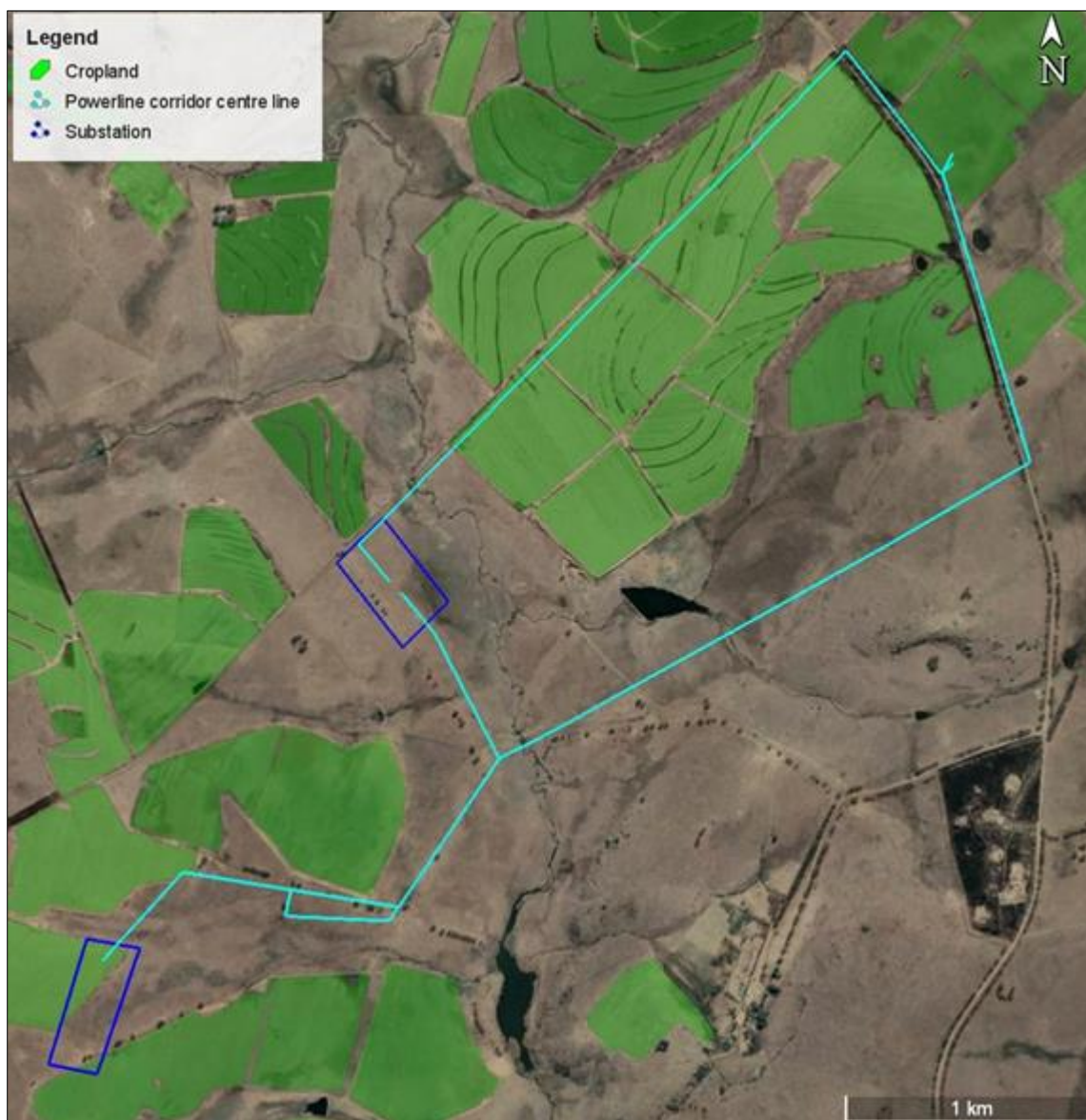
Figure 6-8: Satellite image map of all proposed alternative powerline routes (light blue lines) and alternative substation sites (dark blue outlines)
