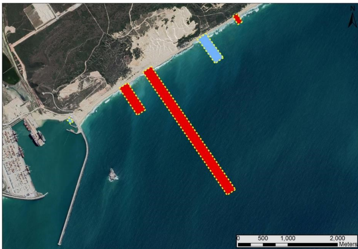
Figure 2.1: Broad locations of the proposed seawater intake (BLUE) and effluent discharge (RED) marine servitudes.
