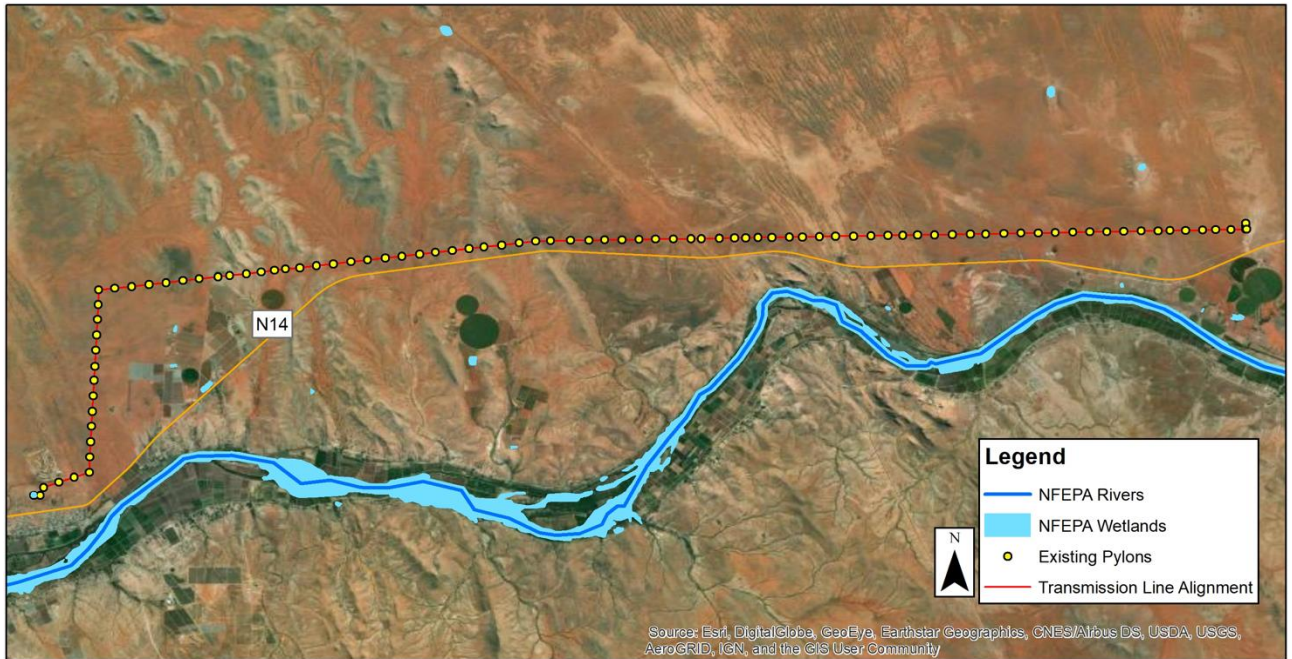
Figure 4-4: Map illustrating the centre line and existing positions of the Gordonia-Avondale 132 kV transmission line pylons. The new monopole structures will be constructed along the existing centreline.
