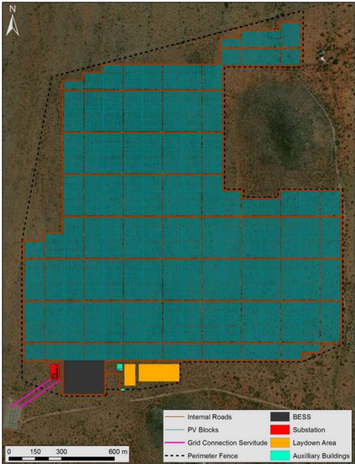
Figure 1: Showing the proposed location of the BESS within the authorised footprint of the facility.
