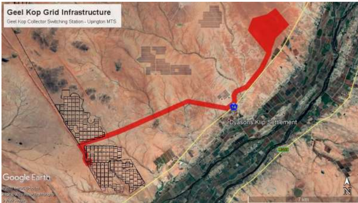
Figure 9: 132 kV line from the Geel Kop collector switching station to the Upington MTS (Preferred) is approximately 16km in length.
