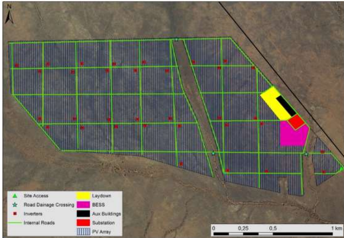
Figure 2: Site Layout plan, showing the proposed position of the BESS (pink polygon) within the authorised footprint.
