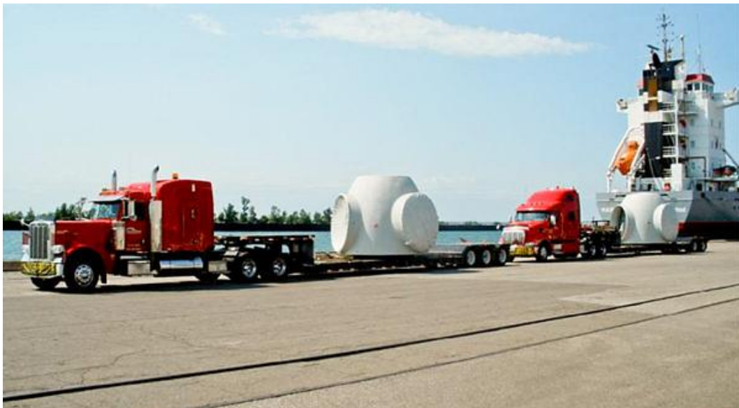
Figure 2.13: Example of a hub and rotary units being transported (Source: Google Images, 2022)
