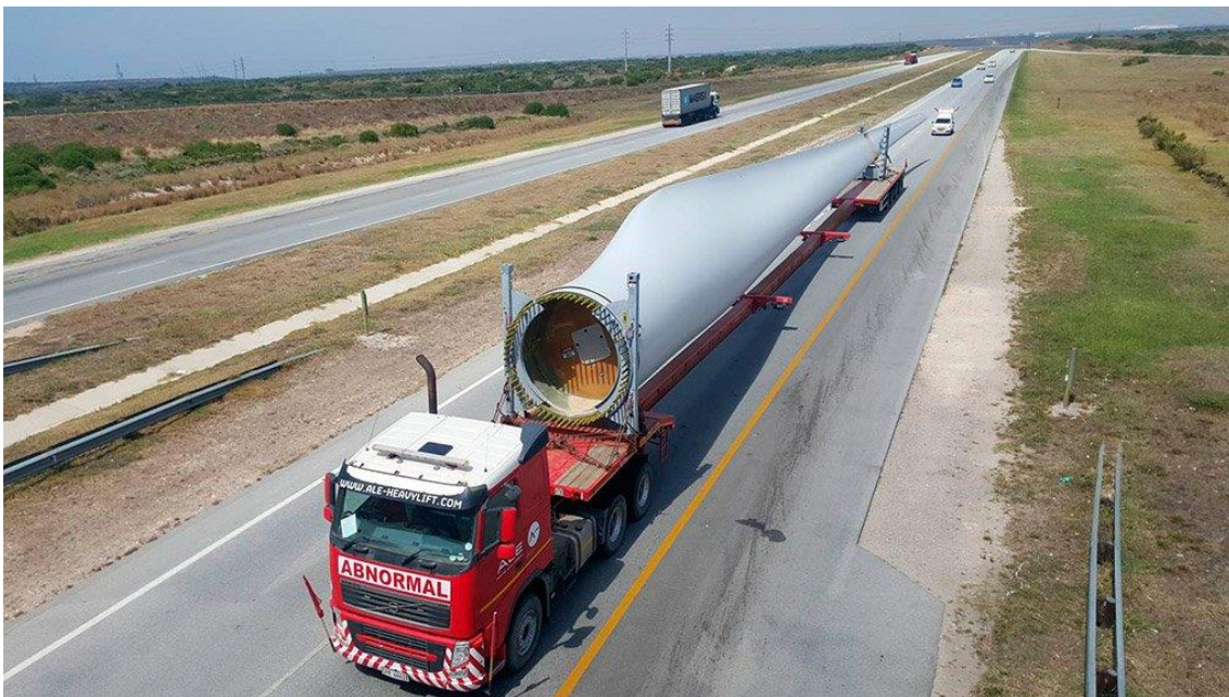
Figure 2.11: Example of a wind turbine blade being transported on an extendable trailer (Source: Google Images, 2022)
