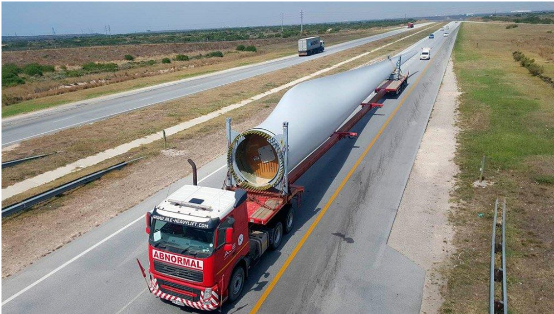
Figure 2.11: Example of a wind turbine blade being transported on an extendible trailer (Source: Google Images, 2022)
