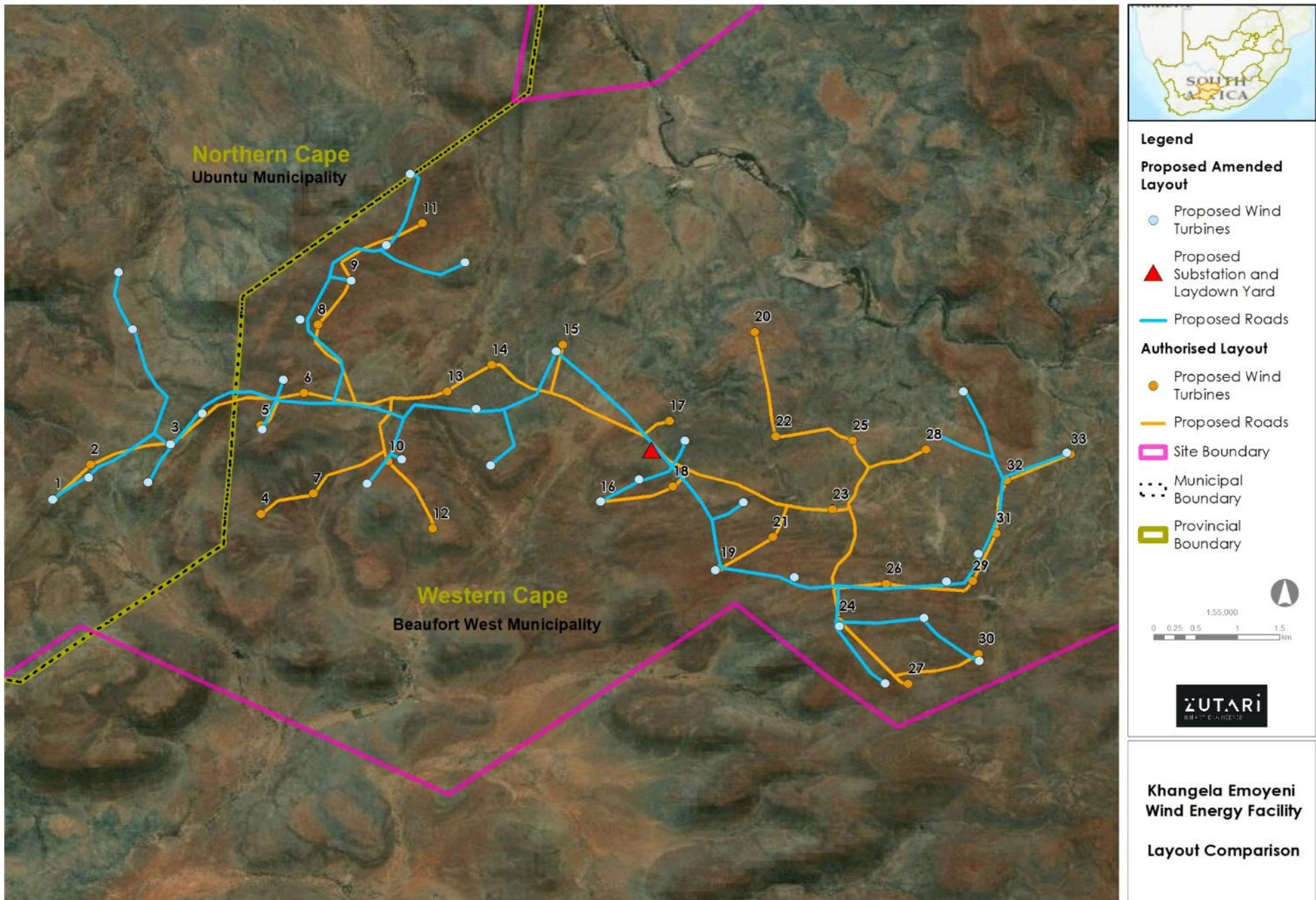
Figure 7: Layout comparison between the authorised (2018) and amended layouts (2020) for Khangela Emoyeni WEF
