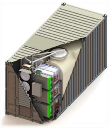
Figure 3-6 Typical Storage of Flow Batteries
