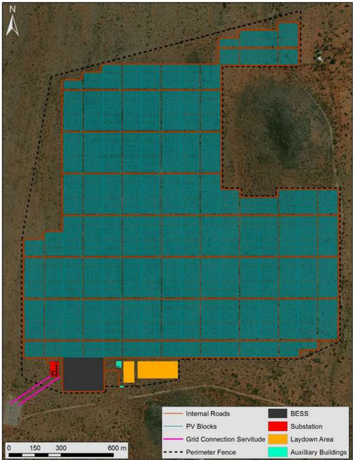
Figure 3: Location of the proposed BESS within the Authorised Footprint of Postmasburg Solar Energy Facility 2.
