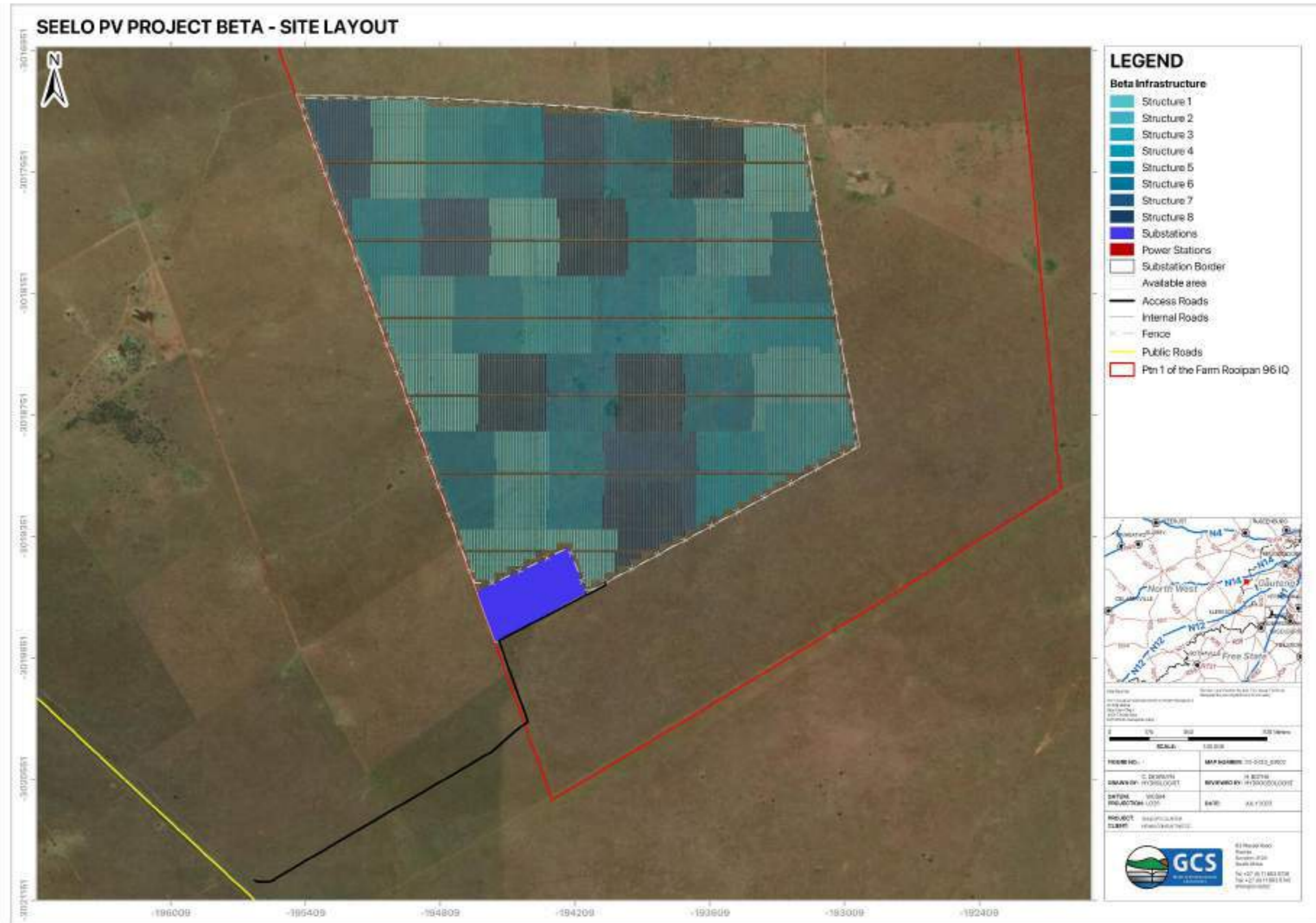
Figure 1-2: Beta PV plant infrastructure and layout
