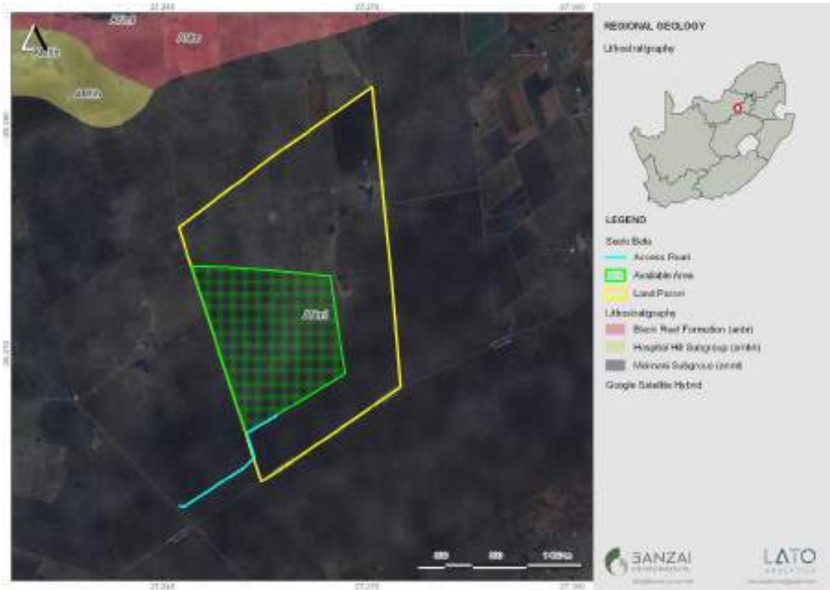
Figure 5: Updated Geology (Council of Geosciences) indicates that the proposed Seelo Beta Solar PV development and associated infrastructure is underlain by the Malmani Subgroup (Chuniespoort Group, Transvaal Supergroup).
