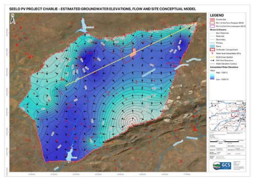
Figure 48: Estimated groundwater depth and flow directions (Botha, 2023).
