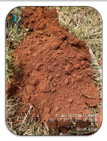
Figure 6: Orthic, red apedal B, unspecified, Hutton soils sampled within the proposed footprint of Seelo Charlie Solar PV
