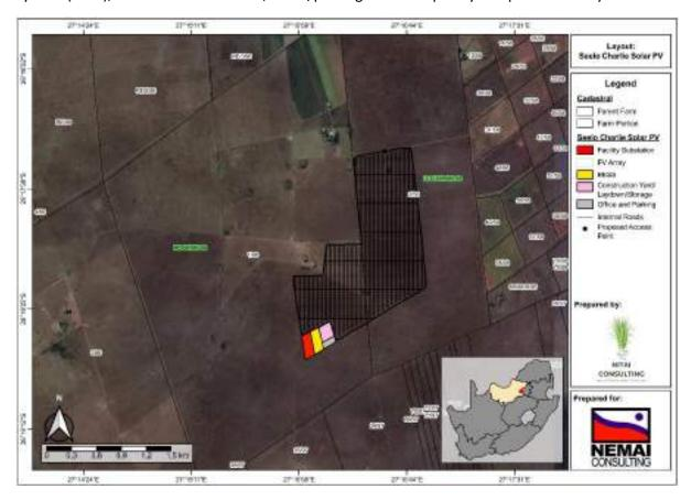
Figure 7: Layout of the Seelo Charlie Solar PV Facility
