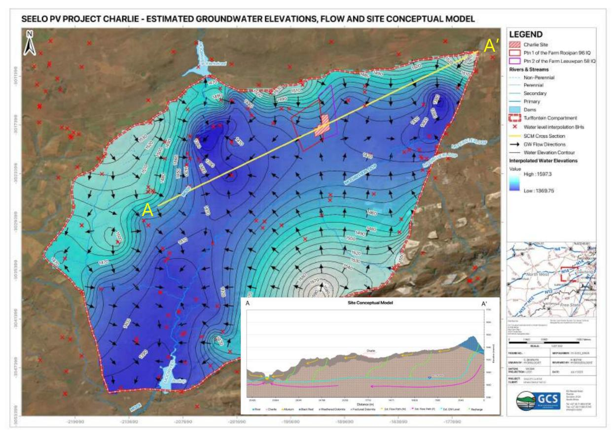
Figure 5-4: Estimated groundwater depth and flow directions
