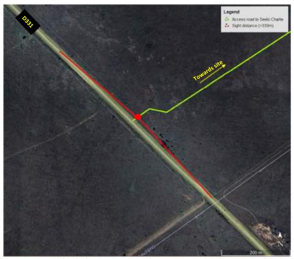
Figure 4-5: Required Sight distances at proposed access point on D331
