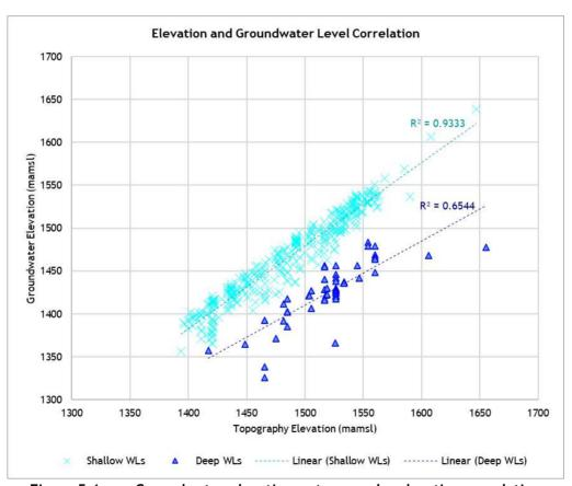
Figure 5-1: Groundwater elevation vs topography elevation correlation
