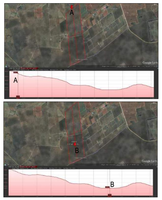
Figure 4: Elevation Profile (maximum elevation at point A and minimum at point B)
