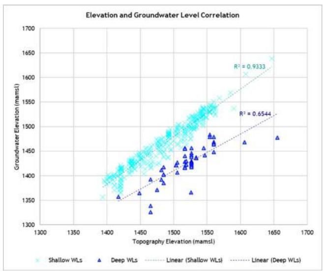
Figure 47: Groundwater elevation vs topography elevation correlation (Botha, 2023).
