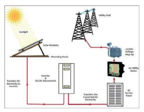
Figure 1:Overview of the solar power plant
