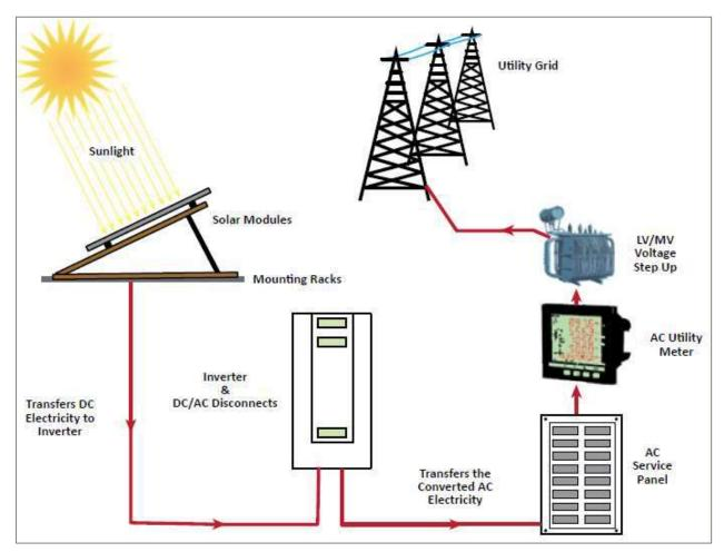
Figure 7: Overview of Solar PV Power Plant (IFC, 2015).
