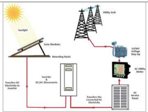
Figure 1: Overview of Solar PV Power Plant
