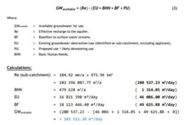
Figure 49: Groundwater balance and reserve determination calculations (Botha, 2023).
