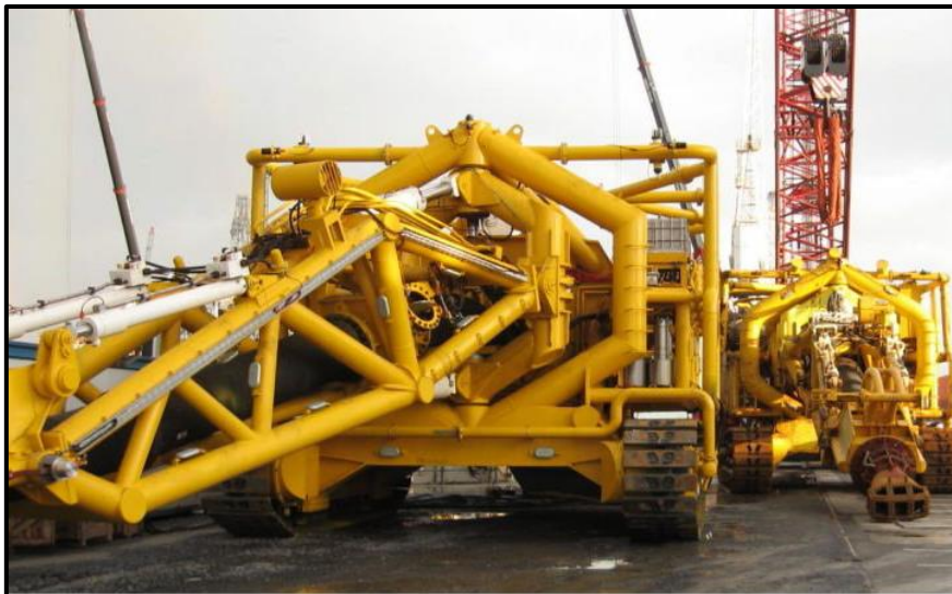
Figure 21: Example of a track-mounted sub-sea crawler
