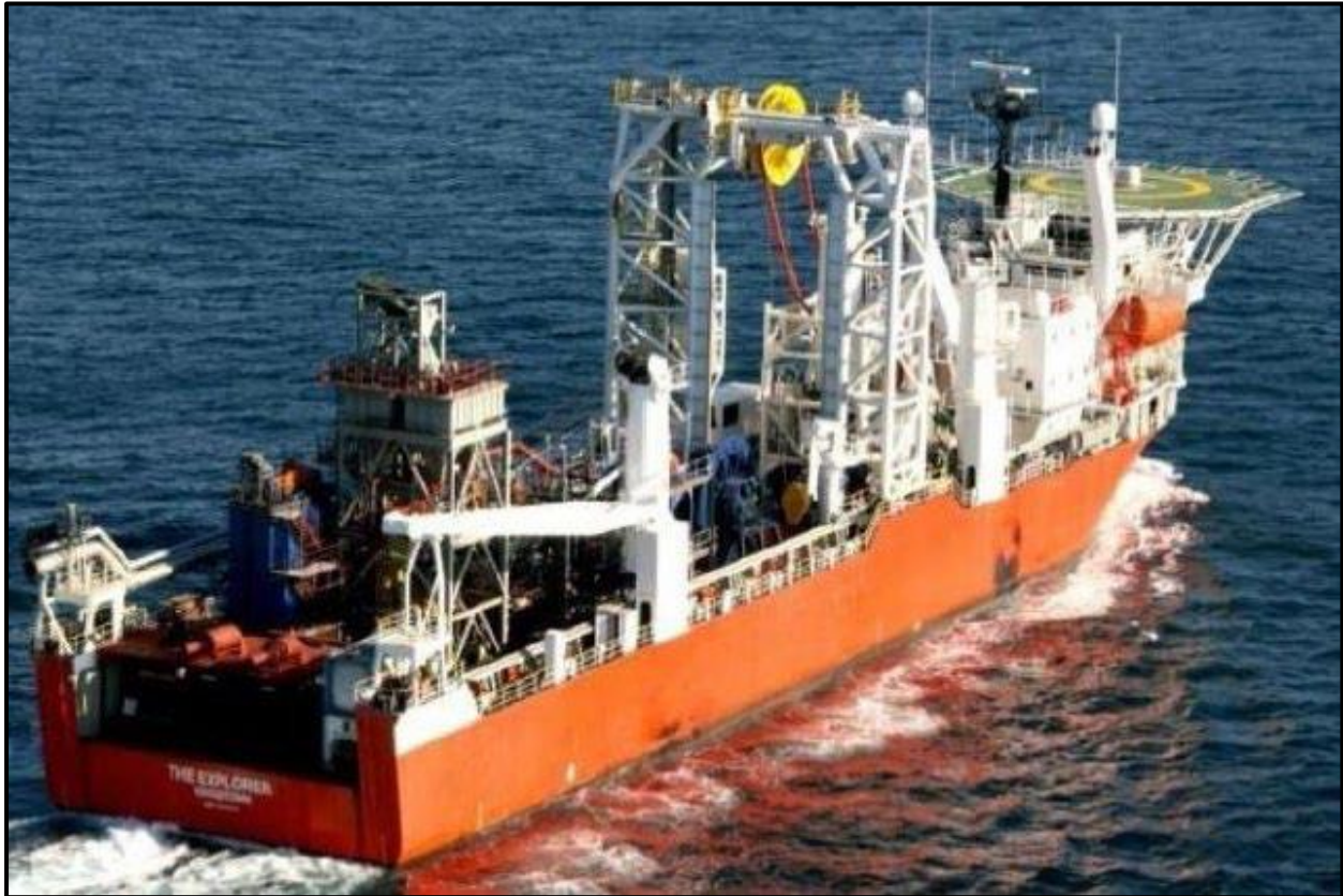
Figure 7: Example of a dedicated drill sampling vessel
