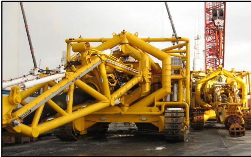
Figure 10: Example of a track-mounted sub-sea crawler
