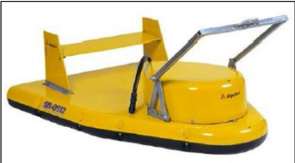
Figure 15: An example of a sub-bottom profiler. Source: Seatronics
