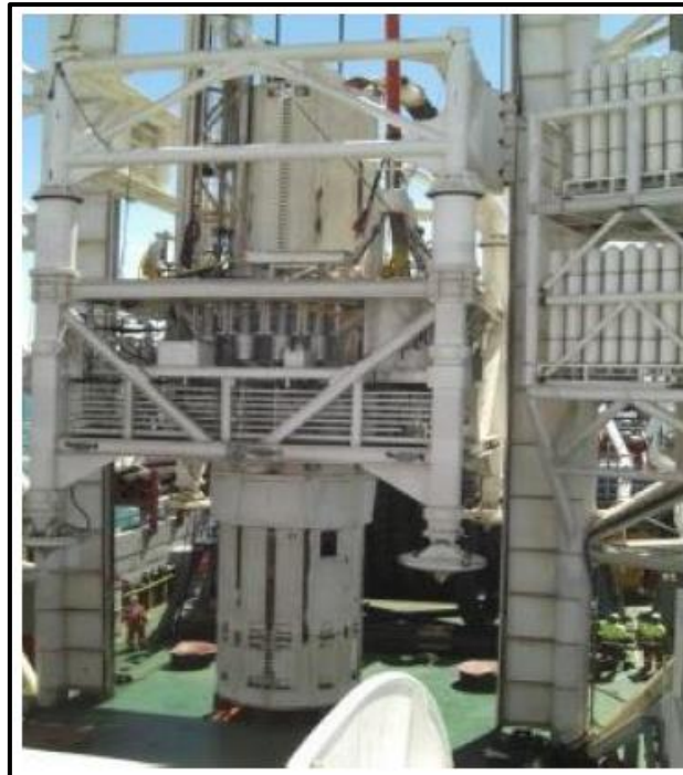
Figure 19: Example of the 2.5 m diameter drill bit within the drill frame structure
