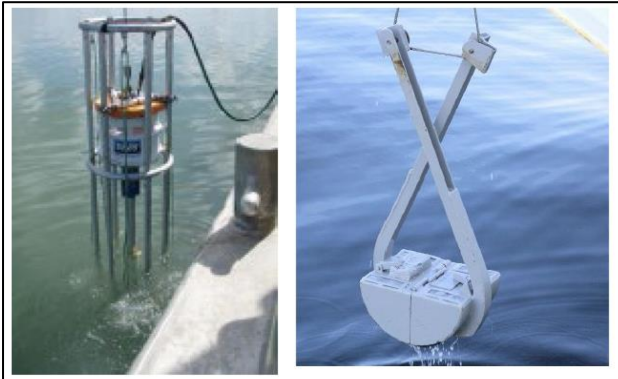
Figure 5: Left Example of a corer and right a Van Veen grab that works like a claw to grab sediment from the seafloor
