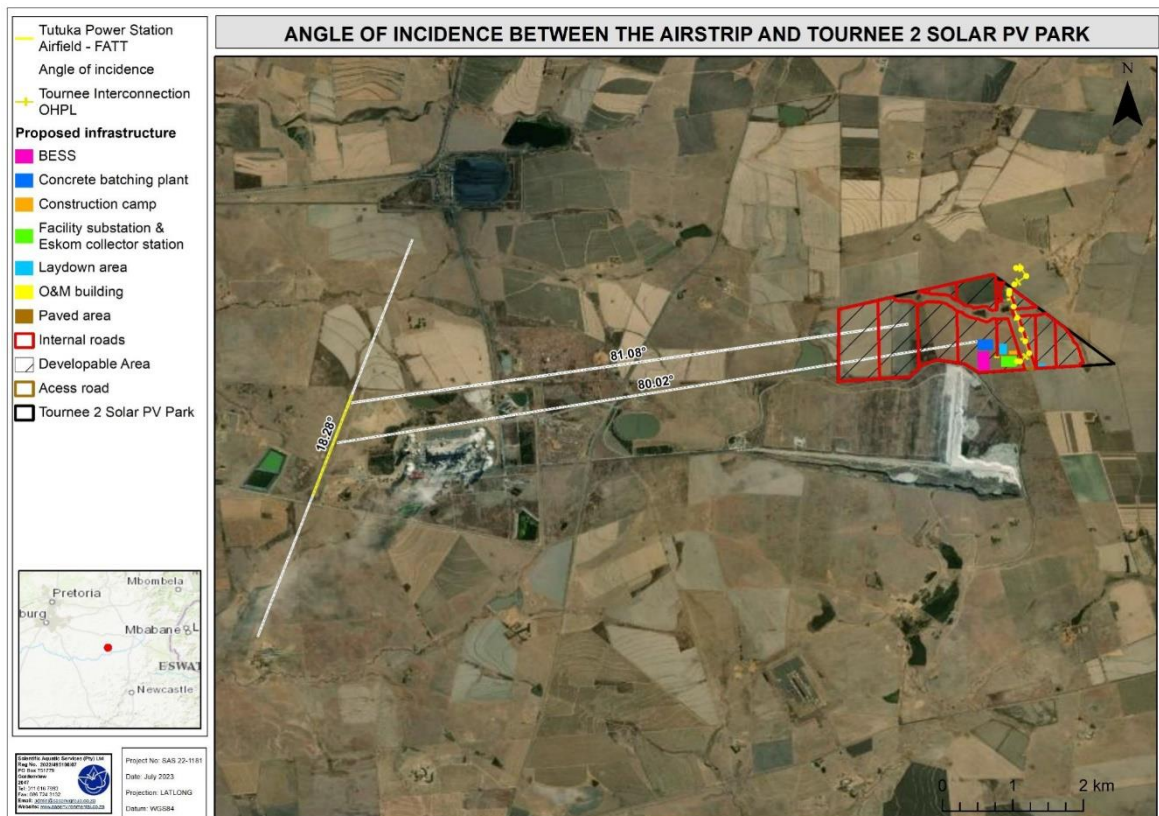
Figure 8-18 - Map illustrating the angle of incidence between the Tutuka Power Station Airfield – FATT and Tournée 2 Solar PV Park, for illustrative purposes.
